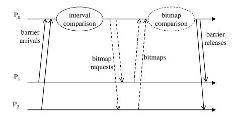
Figure 3. The barrier algorithm has the following steps: 1) read and write notices are sent to the barrier master, 2) the barrier master identifies concurrent intervals with overlapping page access lists, 3) bitmaps are requested for the overlapping pages from step 2, and 4) bitmap comparisons are used to identify data races. Dotted lines indicate events that occur only if sharing is detected in step 2.
