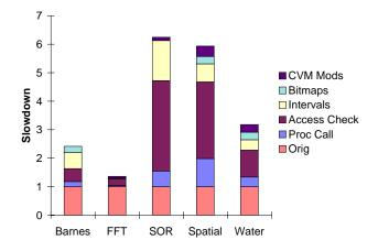
Figure 5. Breakdown of overhead for unoptimized instrumentation techniques.
